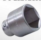
46<sub>mm</sub>, 6-Point thin-wall socket, 3/4" drive. For R & R of front wheel bearing retainer nut on BMW E24, E28, E32 & E34 Chassis.
