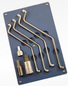
Includes 7mm, 8mm, 9mm & 11mm brake bleeder wrenches, 3 brake caliper sockets & custom powder-coated metal organizer tray. Wrenches fit bleeder screws on Mercedes. BMW. Volvo & VW/Audi models. Applicable to: Brake caliper bolts on the majority of BMW models, Mercedes S-Class (221), newer C-Class (204), M-Class (164); Volvo cars, & rear caliper bolts on 2006-newer VW Jetta & Passat.
