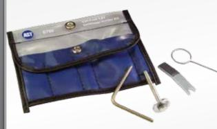
Set contains the #6700-1 Tensioner Bolt & Washer, the #6700-2 Tensioner Locking Plate, the #6700-3 Tensioner Lock Pin & the #6700-4 Holding Rod. Used for holding the timing belt tensioner & the accessory belt tensioner. Applicable to: VW & Audi models w/ a 1.8 Turbo Motor.
