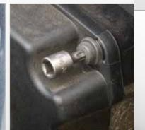
This tool is used to access the door handle fasteners on some Mercedes-Benz models. Applicable to: newer VW Golf, Jetta, Beetle & Passat & 2001-2004 C-Class w/ 203 chassis
