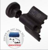
Used to lock the crankshaft in place during timing belt replacement on 2004-2005 VW TDI Pumpe Duse. Used in conjunction w/ #3359, #H 2587-1 & #T 10115.
