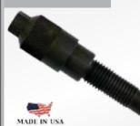
Crank lock pin used to lock the crankshaft at TDC position when replacing the timing belt. Applicable to: Audi 3.0L V6 5V. Used in conjunction w/ **#T 40011**, **#T 40028** & #**T 40030**.
